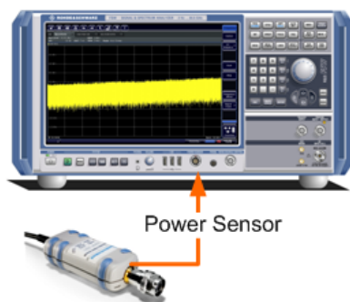
Fig. 5-2: Connecting a power sensor using the POWER SENSOR interface
